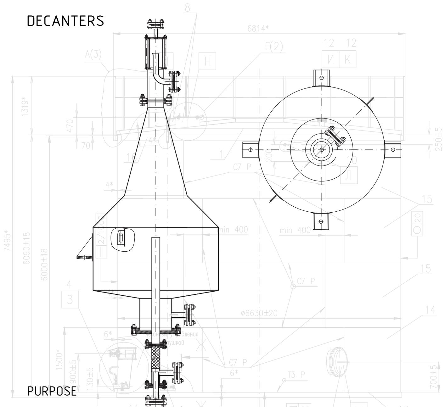
Decanters - technological tanks for storing products of production, are a necessary element of the BRU rectification plant.
